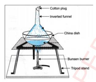
The given figure demonstrate the sublimation process, which one of the following can be separated by this apparatus. **[01]**
