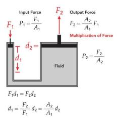
Pressure on the piston of the small area a is given by:
