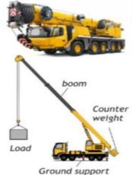
object that is lifted. The counter weight exerts a torque on the crane in equal and opposite direction to the torque from the load. Mathematically,
